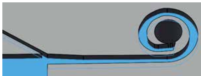
Figure 3. Showing the groove (in blue) in the pre-curved MH electrode mold that cannot be extended beyond one full turn.
