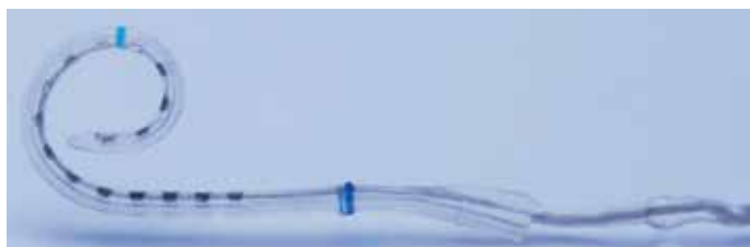
Figure 3. HiFocus Mid-Scala electrode showing the pre-curved shape to conform to the cochlea. It is straightened using a stylet that is removed during insertion.
