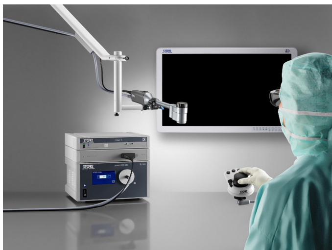
Figure 1. The 3D Exoscope setup and equipment, the Versacrane, 4K monitor, and S Connect are depicted. The surgeon wears 3D polarization glasses. Source: Karl Storz.
