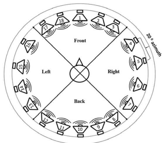
**Figure 1.** Schematic representation of loudspeakers setup for localization testing.
