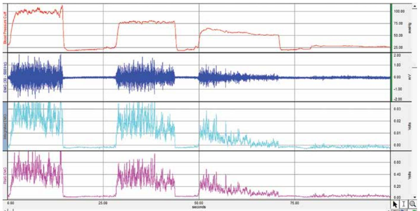
**Figure 1.** The results screen of the Biopac Student Lab PRO program. The upper part shows the generated pressure in the cuff, followed by EMG traces and the root mean square (RMS) EMG in the bottom part.
