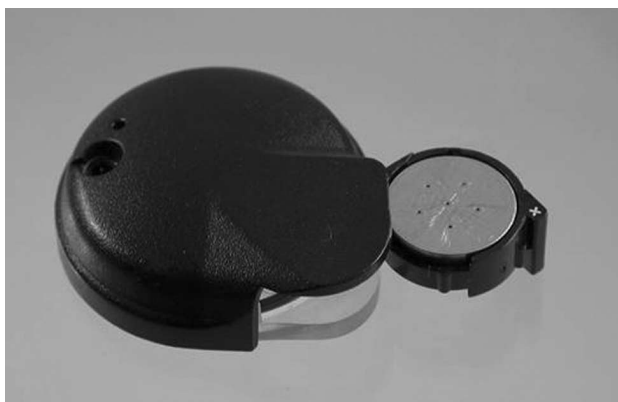
Figure-5: The audio processor (an external part of the VSB) contains a microphone, a signal processor, telemetry electronics, a magnet, and a battery.
